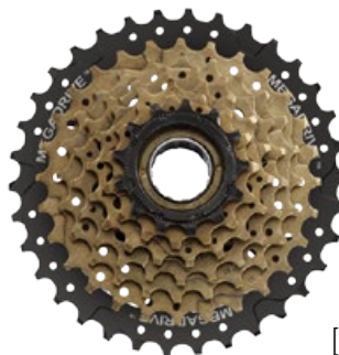
U[Zinc] B[Black] CSM40 7AV 11-34T 7AS 11-28T 7BV 12-34T [7-Speed] [Lightweight Design] U[Zinc] / B[Black]
