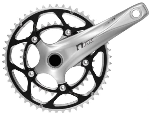
FCRX6 [D1] 50-34T X7 [D1] 50-36T [BCD 110mm] [10-Speed] [6061 Forged Alloy Crank] [Chromoly ISIS Axle] [7075 Chainrings] [7075 Bolts & Nuts] [7075 Axle Bolt] 944~956g [incl. BB] FCRX1 [D1] 53-39T X3 [D1] 52-39T [BCD 130mm]
