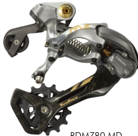
RDMZ80 MD [12/11/10-Speed] MD[1x ≤ 50T, 2x ≤ 42T] [Adjustable Chain Stabilizer] [Carbon Cage] [Forged Alloy Links] 267g
