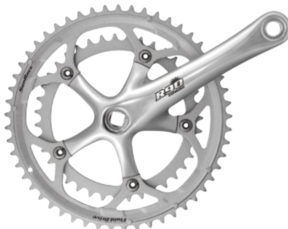
FCR96 50-34T FCR910 53-39T [9-Speed] [SCM435 Bolts & Nuts] [6061 Forged Alloy Crank] 831g[96] / 889g[91]
