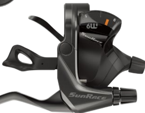
STM930 R9/LL [Dual Release Shift] [Alloy Large Shift Lever] [Alloy Forged Brake Lever] [2/3 Mode Converter] [Stainless Bolt] [Slick-Stainless Cable] 423g/pair
