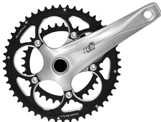
FCRS6 (S1) 50-34T FCRS1 (S1) 53-39T [BCD 110mm] [BCD 130mm] [10-Speed] [6061 Forged Alloy Crank] [Alloy Chainrings] [7075 Bolts & Nuts] [7075 Axle Bolt] 944~949g [incl.BB]
