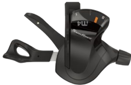
DLM400 R8/R7/L3 [Dual Release] [Composite Levers] [SCM435 Bolt] [Slick-Galvanized Cable]
