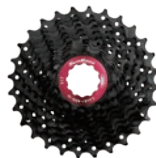
O[Black Chrome] X[Metallic Silver] CSRX1 EAS 11-28T EAU 11-32T EAW 11-36T [11-Speed] [Alloy Spiders] [Alloy Lockring & Spacers] O[Black Chrome] / X[Metallic Silver] 278g[AS] / 290g[AU] / 360g[AW]
