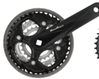
FCM500 42-34-24T [8/7-Speed] [Alloy Forged Cranks] [Square Taper]
