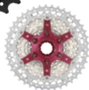
CSMX8 EAZ 11-46T EAY 11-42T EAX 11-40T [11-Speed Wide Ratio] [A7075 Largest Sprocket] [Alloy Spiders] [Alloy Lockring & Spacers] O[Black Chrome] / X[Metallic Silver] 465g[AZ] / 401g[AY] / 389g[AX]
