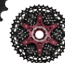
CSRX8 EAX 11-40T EAY 11-42T [11-Speed Wide Ratio] [A7075 Largest Sprocket] [Alloy Spiders] [Alloy Lockring & Spacers] [For 11-Speed Road Hub] O[Black Chrome] / X[Metallic Silver] 392g[AX] / 404g[AY]
