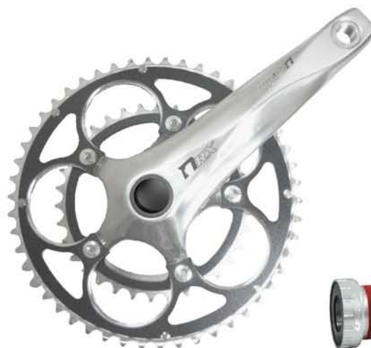
FCRX6 [D1] 50-34T X7 [D1] 50-36T [BCD 110mm] FCRX1 [D1] 53-39T X3 [D1] 52-39T [BCD 130mm] [6061 Forged Alloy Crank] [Chromoly ISIS Axle] [7075 Chainrings] [7075 Bolts & Nuts] [7075 Axle Bolt] [885~927g incl. BB]
