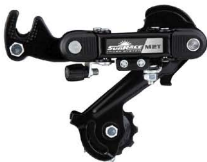
RDM2T LD/LB SD/SB [7 & 6-Speed] [Index Cable Adj.]
