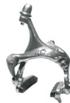
BCRS F/R/P [Quick-Release] [Forged Alloy Caliper] [Cartridge Brake Shoe Pads] [Convex Washer Adj. Shoes] [184g]
