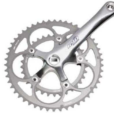
FCR9F 50-34T FCR9A 53-39T [Alloy Chainrings] [SCM435 Bolts & Nuts] [6061 Forged Alloy Crank]
