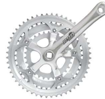
FCR96 50-34T FCR97 52-42-30T FCR91 53-39T [SCM435 Bolts & Nuts] [6061 Forged Alloy Crank]
