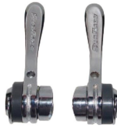
SLR63 Braze on: R8/LF B[28.6mm] C[44mm] Clamp: 8F H[22.2mm] G[25.4mm] D[28.6mm]
