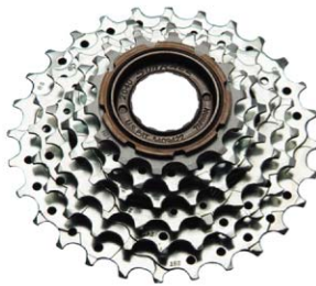
MFM22 6DS 14-28T U[UCP] [Lockring Design] [Light Weight Design]
