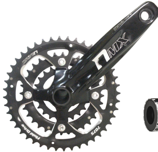
FCMX7 44-32-22T [6061 Crank] [Chromoly Axle] [7075 Chainrings] [7075 Bolts & Nuts] [779g incl. BB]
