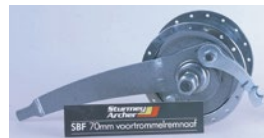
1977 SBF 70mm Front Drum Brake
