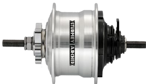
RX-RK5 5 Speed Disc Brake Hub
