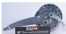
1977 SBF Front Drum Brake
